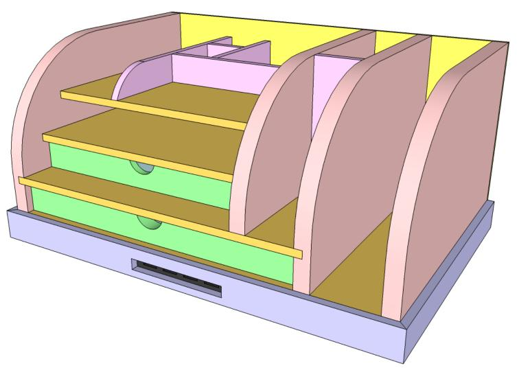
Note: this design features only two drawers and a USB hub in the middle. I eliminated the mitered cotners on the molding and drawers. I also eliminated the rabbets on the drawers to hold the drawer bottoms.
